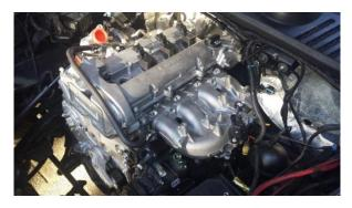
The spark-ignition engine running on LPG
